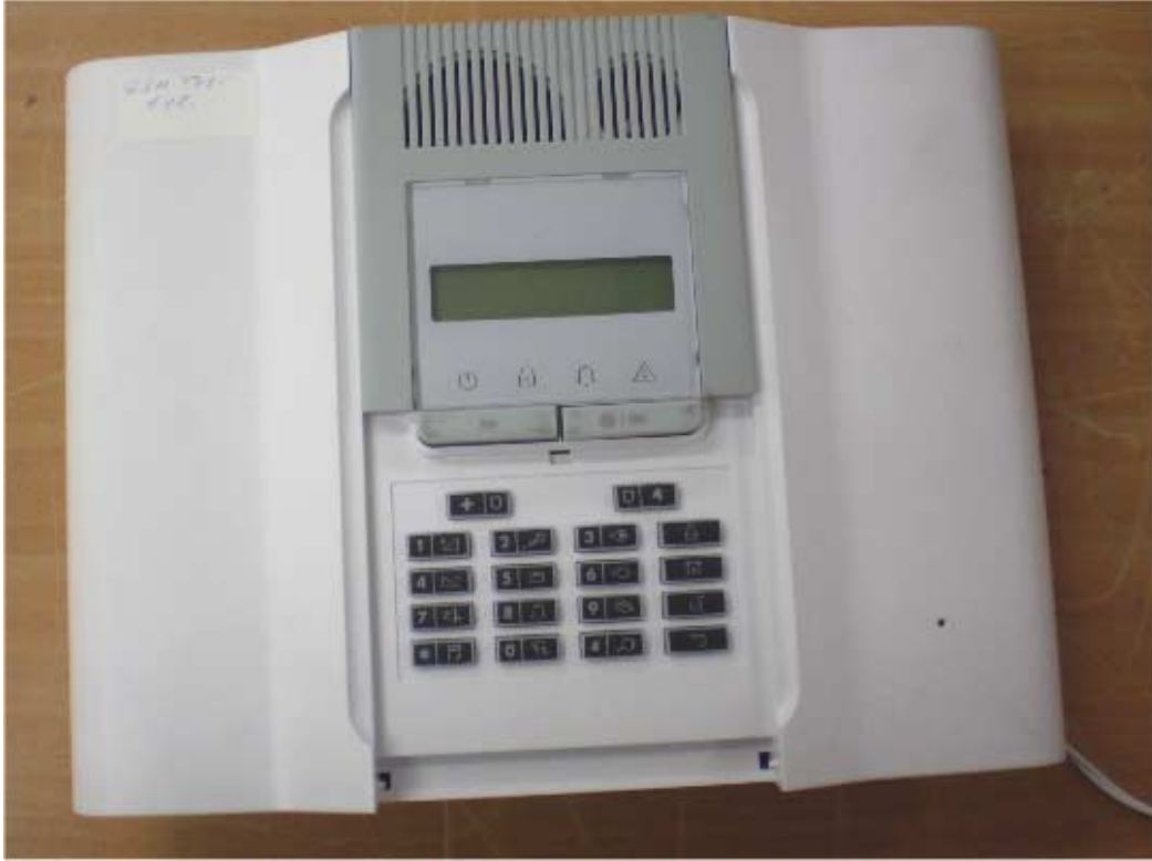
Photograph No.1 PowerMaxComplete general view
